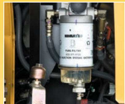
Fuel pre-filter with water separator
